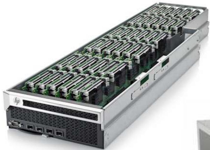
An HP Redstone server tray crammed with Calxeda ARM servers (** total of 72 server nodes)
